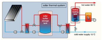
The solar support of process steam generation is usually only economical when a significant part of the steam is used in the processes directly (the steam network is an open or partly open system). Solar heating of the additional, demineralised make-up water can be attractive; heating of the condensate return flow or the feed water directly is more expensive because of the high temperatures. Additionally, at state of the art installations the feed water is usually preheated by an economizer.
