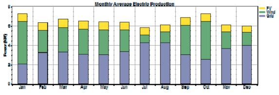
Figure 27: Monthly average electricity production from the proposed system
