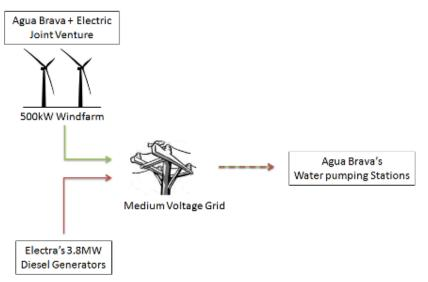
Figure 5: Electricity usage scheme of the proposed project
