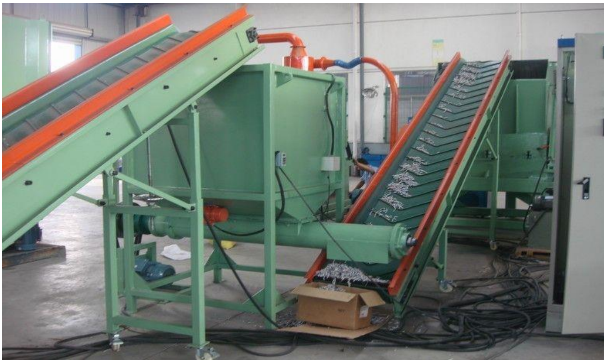
Automatic cable granulator ( http://www.cable-recyclingmachine.com/ 2015)
