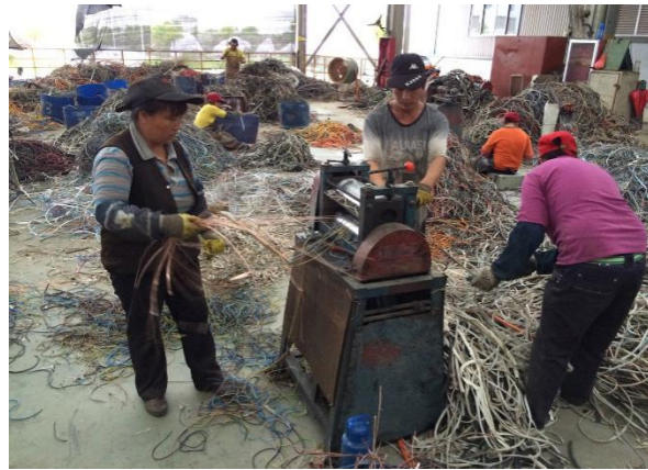
Semi-mechanical wire stripper (Sofies 2015)
