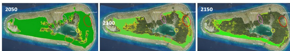
Figure 3. SLR Inundation modelling for Vaitupu (no waves, green shows area above high water mark) (Source: Arthur Webb)
