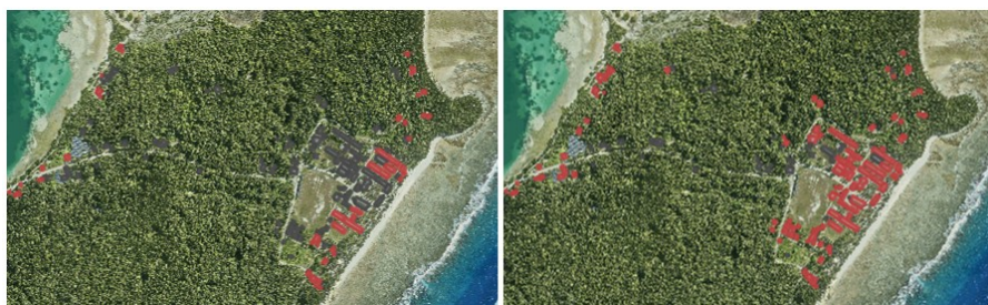
Figure 5. Buildings at risk from 1 in 5 year flooding event between current (left) and 2060 (right) under the SSP2-4.5 climate change scenario. The cluster on the left of each image shows the clinic complex, and the right shows the secondary school. Red shapes denote buildings at risk of flooding (Source: Tuvalu Coastal Adaptation Project - TCAP )
