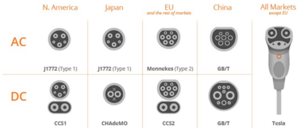
Figure 3 AC and dc ev charging standards around the world (SOURCE: enel x)
