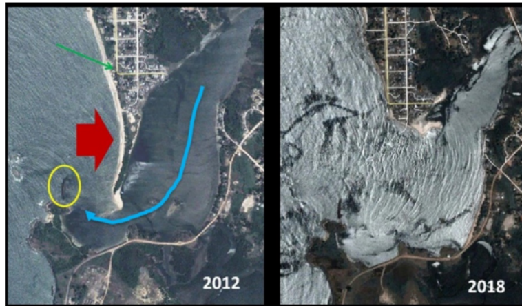
Figure 1. Satellite photos of the Sinoe River delta in Greenville taken in February 2012 (left) and March 2018 (right) show sizable erosion of the Greenville peninsula area resulting in more than 50 houses being eroded or incapable of further habitation (red arrow). In addition, the southern tip of the main Mississippi Street and side streets (green arrow) have been completely eroded. The blue arrow represents the main river current direction along the original riverbed. A shipwreck (from 1990s civil war) at the mouth of Sinoe River delta has been encircled yellow and is believed to possibly have a function in redirecting local ocean bay currents towards the Mississippi Street area, which will be exacerbated by projected climate changes including an increased frequency of high-intensity rainfall events[52] 52 .
