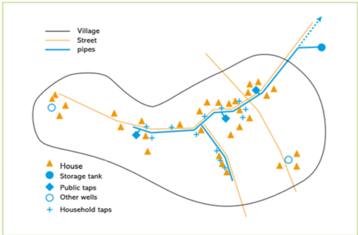
Figure 4 – Scheme of village's water supply system
