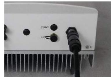
▲ Figure 4.16 Connect AC Terminal Connector to the inverter
