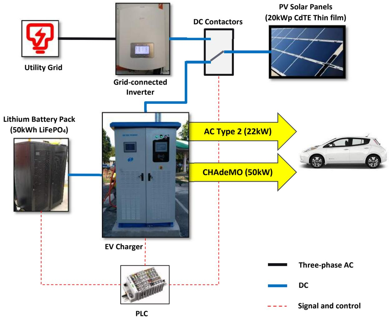
Figure 1 Overview of the components in the installed PV-based EV charger with energy storage system
