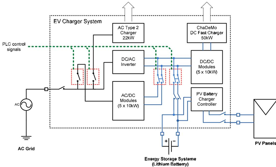
The EV Charger System consists of several main subcomponents as shown in the figure above. The AC (three-phase four wires) connections are given in black, DC connections are given in blue and the control signals (from PLC) are given in green.
