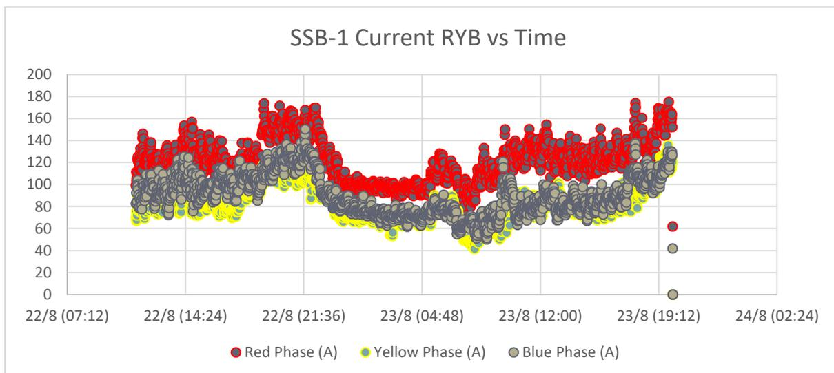
Figure 8 Logged three-phase current at SSB-1.
