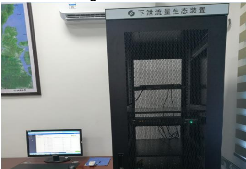
Ecological flow monitoring system
