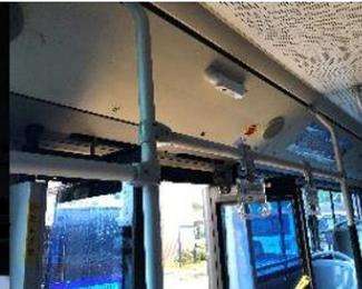
Passenger flow counting device deployed on buses in Suzhou
