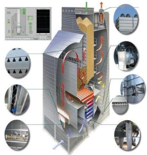
Cut section diagram of the LSU dryer
