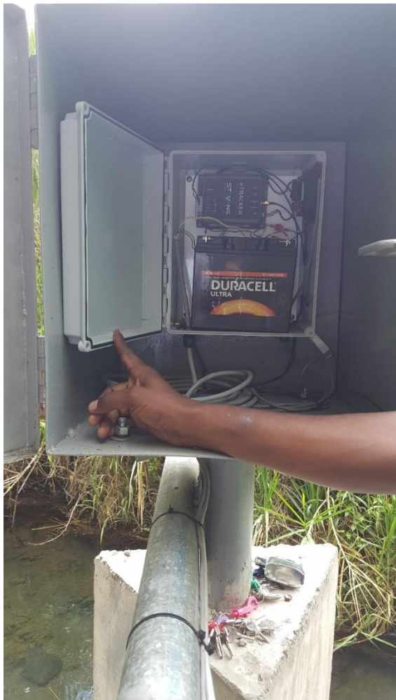
WRA Stream flow station installed on the Hope River
