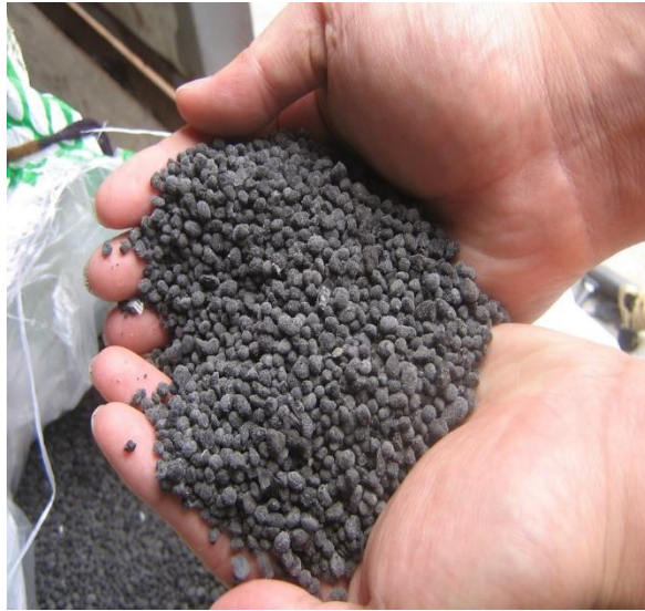
Fig 2. Biochar compound fertilisers are a mixture of biochar, chemical fertilisers and binders
