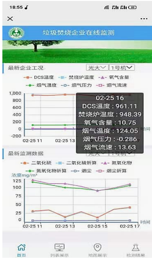
Figure 13. Ningbo Incineration Operating and Emissions Data Accessible on Mobile App
