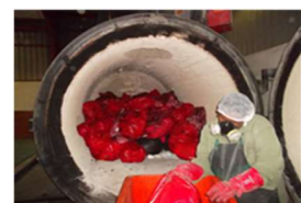
Figure 2024 Bad practice-loading an incinerator from front door
