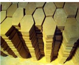
Figure 16 Production of bricks from recycled plastic
