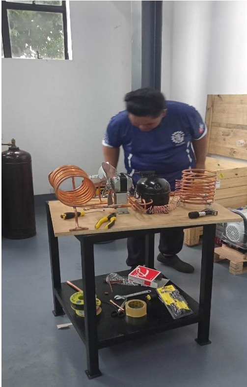
The participants fabricating a simple R290 simulator
