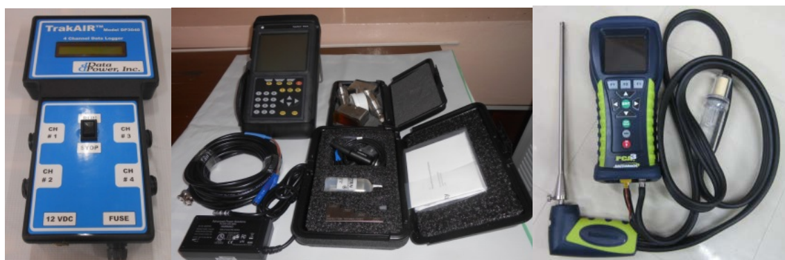
Figure 6. Data logger for compressed air (left), flow meter for pump (center), and combustion analyzer for steam (right)
