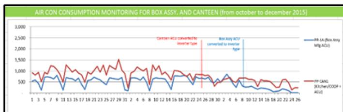
Another initiative was to replace the conventional AHU units to energy efficient systems. The savings graph below illustrates the use of data to substantiate the energy savings achieved.
