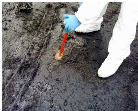
Figure 12: Sampling of soil and transformers
