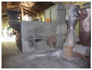
One of the facility's two incinerators, the waste is fed through the access door in the centre of the picture.
