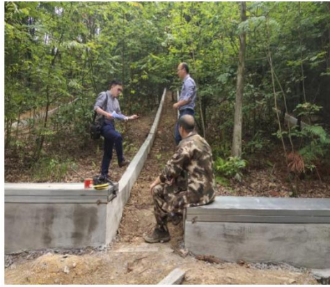
Figure 13: Monitoring runoff field of water and soil conservation in Gonglongping SFF in Guizhou
